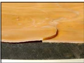
**Delamination** – Linear polyethylene is a thermoform plastic, which means it can be melted and cured multiple times. Crosslinked polyethylene is a thermoset plastic, which means the cure is permanent, and cannot be reset. The two plastics do not permanently bond. In application, the sidewall expansion and contraction caused by a tank being filled and emptied creates further long-term stress on the two materials' seam. As a result, end users have experienced delamination failures.
