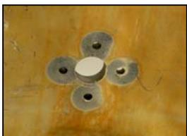
**Fitting and Outlet Chemical Exposure** – Since it is difficult to mold a uniform wall of linear polyethylene within the dual layered tank processing technique, fitting locations often have to be ground down and smoothed over to achieve a uniform sealing surface, which can inevitably result in the removal of the linear layer and the required chemical resistance protection that goes with it.
