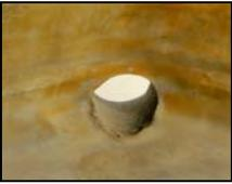
The linear liner protection can also be compromised when holes are drilled into the tank wall removing the chemical resistance barrier and exposing the outer XLPE shell to chemical attack.
