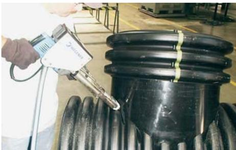
Hot air extrusion welder
