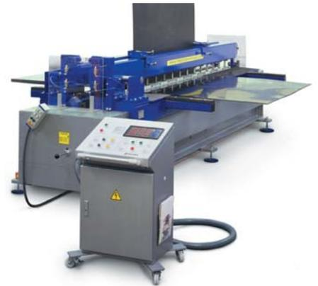
10 ft. butt welder set up for welding of 90° corners.
